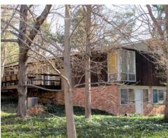
A "banked slope" building with aboveground brick walls that extend from the foundation (recommended).
