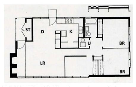
Floor plan of Unit No.2 (c. 1960) with the "U" or utility core at the center of the house. *Hollin Hills, A Community of Vision* (2002), p.50.
